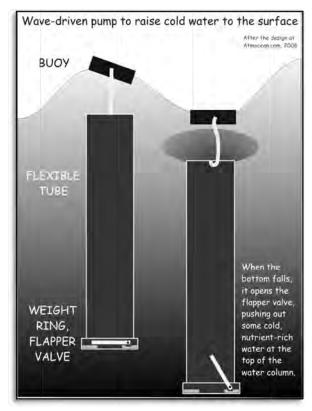
Technology can perhaps mimic the natural upwelling from the nutrient-rich depths in less well endowed regions of ocean surface. Inventors have been busy patenting schemes, despite the lack of money for demonstration projects. One patent is simple enough to explain in one page. I wish I'd thought of it myself. The diagram shows a simple scheme for using the ups and downs of waves to power the uplift of cold, nutrient-rich deep waters.
